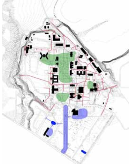
This diagram illustrates documented stormwater pipes & retention areas. Undocumented areas are green.
